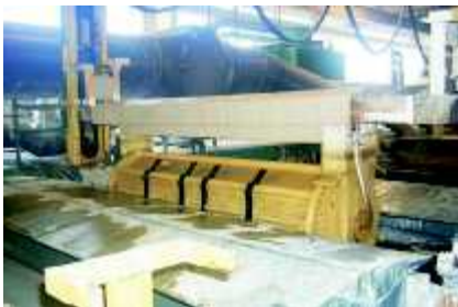
Plating barrel on an auto line lowering into the tank
