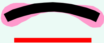
Thin deposit in centre of Concave Surface
