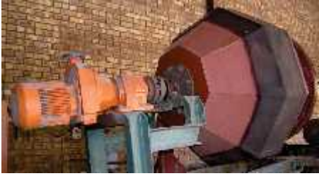
Mechanical Plating tumbler unit at Team Plating Works
