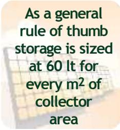
As a general rule of thumb storage is sized at 60 Lt for every m<sup>2</sup> of collector area
